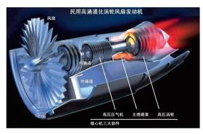
Figure 1. Turbine engine with high bypass ratio for civil use scheme
