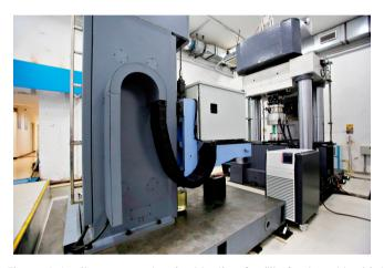
Figure 1. In-situ geomechanical testing facility featured by high energy linear accelerator CT scanning and multi-field coupling
