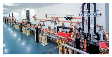
Figure 1. Electron linear accelerator of Dalian Coherent Light Source
