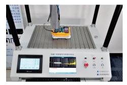
Figure 1. Testing and positioning equipment for basic elements of electromagnetic emissions
